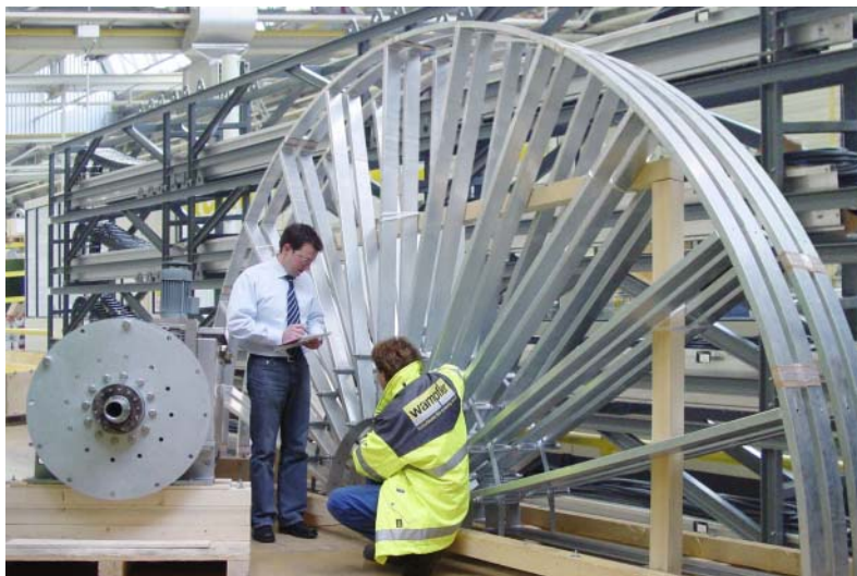
Caption: Final inspection of the energy supply for the Gottwald Port Technology's new crane generation at Wampfler AG in Weil am Rhein.
